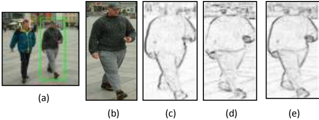
Figure 4: (a) Original Image with Bounding Box and Resized Image. (b) Resized Image (c) Horizontal Gradient (d) Vertical Gradient (e) L1 Normalized Gradient
